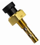
The **S292** is an active device designed to give an alarm signal if liquid falls below, or rises above, a preset level. It can be specified with a delay to eliminate false alarms due to turbulence.
