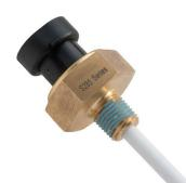
The **\$285** is an active device designed to give an alarm signal if liquid falls below or rise above a preset level. It can be specified with a delay to eliminate false alarms due to turbance. Containing a factory programmable microprocessor, the switch offers sink to ground a reduced risk of damage and a wide range of customer specifiable options make it suitable for most applications.
