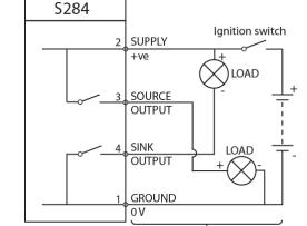
NOTE: IF SINK ONLY OUTPUT IS REQUIRED THEN PIN 3 IS NOT USED.
