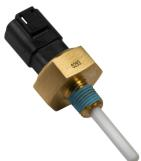
The **S283** is an active device designed to give an alarm signal if liquid falls below, or rises above, a preset level. It can be specified with a delay to eliminate false alarms due to turbulence.
