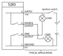
NOTE: IF SINK ONLY OUTPUT IS REQUIRED THEN PIN 3 IS NOT USED.
