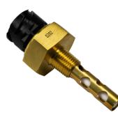
The **5282** is an active device designed to give an alarm signal if oil falls below, or rises above, a preset level. It can be specified with a delay to eliminate false alarms due to turbulence.
