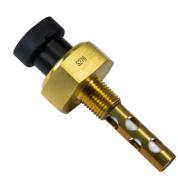
The **S276** is an active device designed to give an alarm signal if liquid falls below, or rises above, a preset level. It can be specified with a delay to eliminate false alarms due to turbulence.
