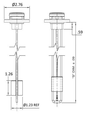
The Rochester magnetic liquid level gauge operates simply by means of a float actuating a powerful magnet inside the container which in turn provides an invisible "magnetic coupling", through a solid head, with the magnet on the pointer in the dial chamber. Thus the gauge head completely seals off the liquid in the container so the dial may be removed and replaced quickly anytime without loss of liquid.
