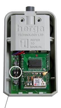
Removing the rear panel gives the user access to switches for setting the latency of the system and sleep timeout of the connected transmitters
