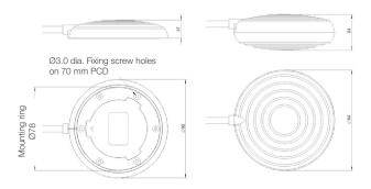
Note: To remove mounting ring from bellows as supplied, insert a 3 mm dia. bar in one of the holes & twist anti-clockwise through 41°. Mounting ring can be used as a template for drilling/tapping holes in mounting face.
