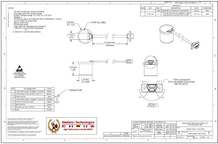
Figure 5 Standard Pigtail with Connector Options for G200 Outline Drawing
