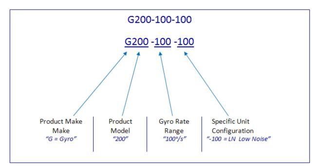
Figure 9: Gladiator Technologies Part Naming Conventions for G200 Dual Axis MEMS Gyros
