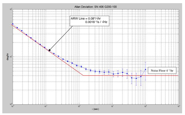
Figure 23 Typical ARW Random Walk Gyro Noise – X Gyro
