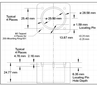
Figure 15: G200 Recommended Mounting Dimensions
