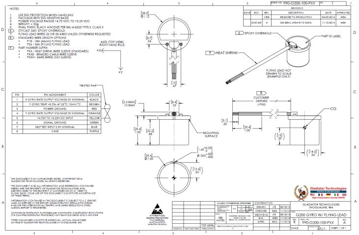
Figure 4 Standard Pigtail Options for G200 Outline Drawing
