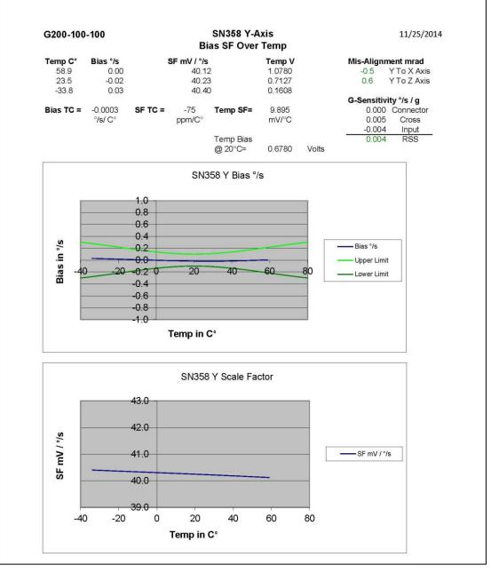
Figure 20 Bias & Scale Factor Over Temperature – Y Gyro
