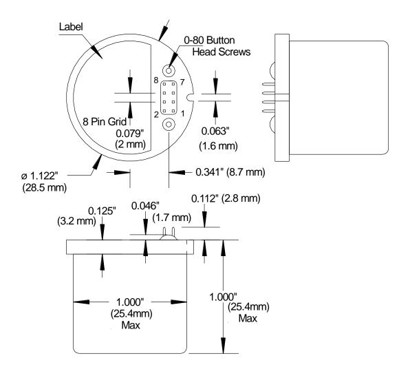
Figure 6: G200 Dual Axis MEMS Gyro Outline Drawing
