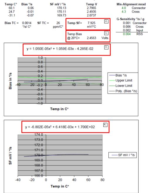
Each gyro is supplied with the Calibration data per the above example. In each chart is the  $2^{nd}$  order model equation for bias in °/s over temperature in C° and for scale factor in mV/ °/s over temperature in C°. Also included is a model for the temperature sensor bias voltage at 20 C°
