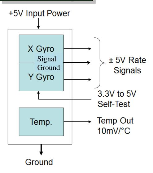
Figure 8: G200 Dual Axis Gyro Block Diagram
