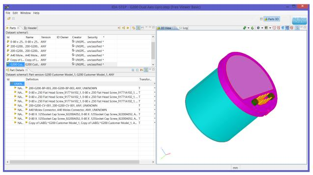
Figure 2 G200 Gyro 3D Model (STEP)
