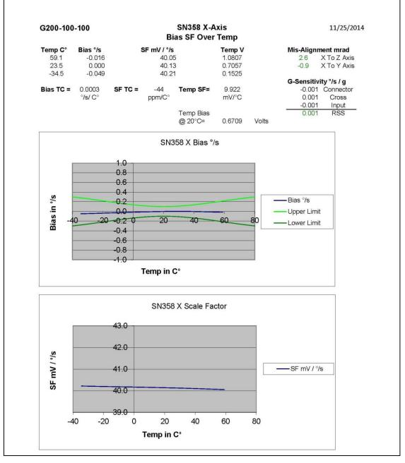
Figure 19 Bias & Scale Factor Over Temperature – X Gyro
