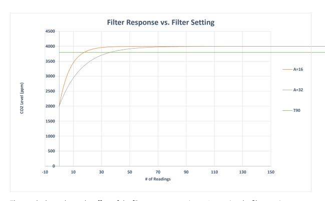
The graph above shows the effect of the filter on response times. Increasing the filter setting increases the measurement output response time.  $T_{90}$  is the time to 90% of reading. The CozIR®-LP3 takes 2 readings per second. The CozIR®-LP3 sensor will also output the raw unfiltered CO<sub>2</sub> measurement data. This data can be post processed using alternative filter algorithms.
