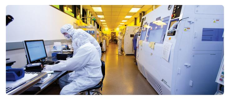
Merit Sensor owns and operates a MEMS wafer fab, which enables the production of customized piezoresistive pressure sensors.
