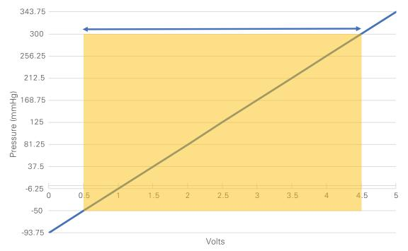
Compound sensor (measuring both vacuum and gage; both sides of zero) Output = 0.5V to 4.5VPressure = -50 to +300mmHg (typical blood pressure applications)
