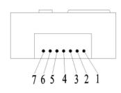
Note: All the pins for reserved must be vacant while the sensor is working.
