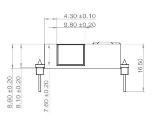
Pin is the common standard type with square cross section.
