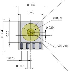
Cap placement tolerance measured  $\neg$  from the cap  $Q_{\perp}$  to the substrate  $Q_{\perp}$ Long axis: .039 Short axis: 0.0
