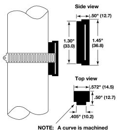
**BDS** Sensor Dimensions Non-invasive strap-on sensor inches (mm)
