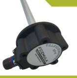
The **T/LL312** series of advanced sensors is designed to continuously monitor the contents of a tank in extreme temperature applications such as defence and off-highway vehicles. Capable of operating at temperatures between -40°C and +125°C, the sensor auto compensates when a liquid with a different dielectric constant is used. For example, if it is used in a tank of conventional diesel, the user can refill with bio-diesel and the sensor will correct the output level automatically.
