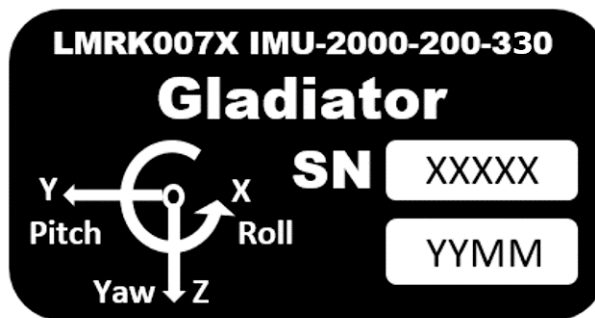
Figure 1: LMRK007X IMU part label with axis definitions, serial number, and date code of manufacturing.
