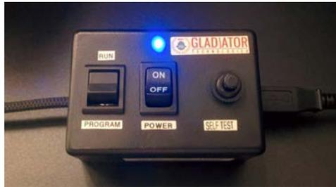
Figure 13 Self-Test, Power, and Run/Program
