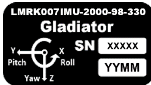
Figure 1: LMRK007 IMU part label with axis definitions, serial number, and date code of manufacturing.
